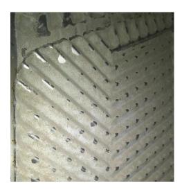
The heat exchanger was opened for inspection of the plates 10 months after installation of the conditioning system. These pictures, taken as soon as it was opened and had not been maintained or washed yet, show the condition of both sides of the plate. Our client noted they are extremely clean and the small amount of hard water deposits on them flake off easily when touched.
