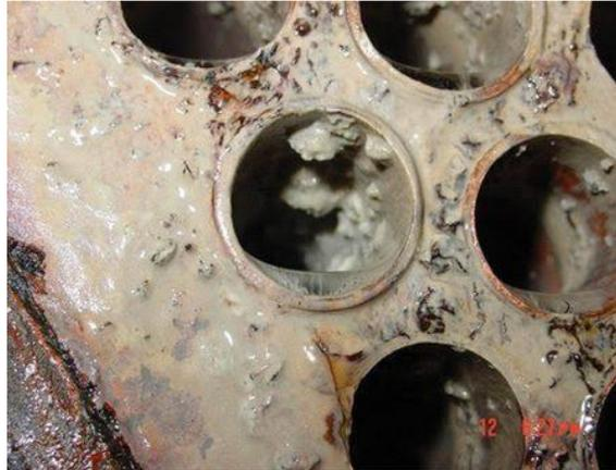
Biofilm on cooling system pipes not only presents a potential health hazard but also drastically reduces energy efficiency.
